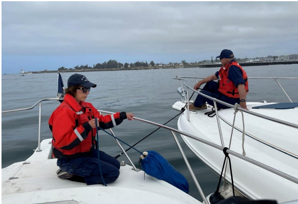
With the #1 line made, Auxiliarist Jane Smith tends a “walking fender” ... a fender that is hand-held and can be placed quickly when and if needed.
