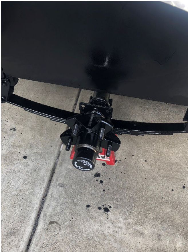
Trailer Bearing Repaired
