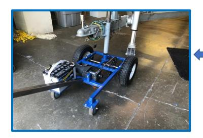
This is a trailer tug John Hardin constructed to move his boat trailer. This tug is similar in concept to the tugs used to push commercial airliners back from their airport gates.
