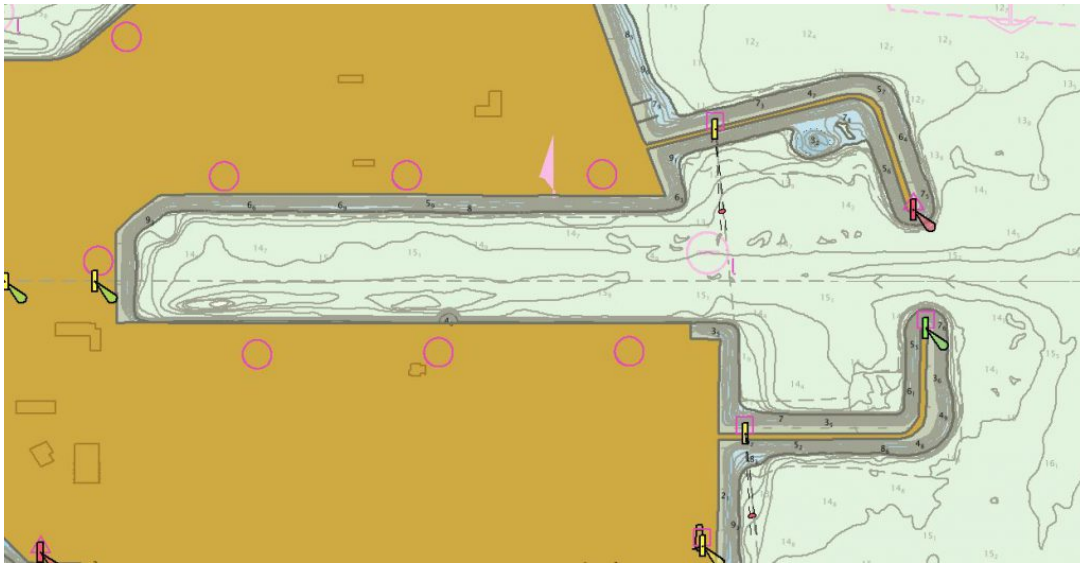
A berth in Los Angeles/Long Beach Harbor depicted on a band 6 (or berthing level ) HD electronic navigational chart.
