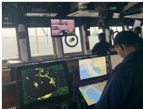
Electronic navigational chart displayed on an Electronic Chart Display and Information System (ECDIS) on NOAA Ship Thomas Jefferson.
