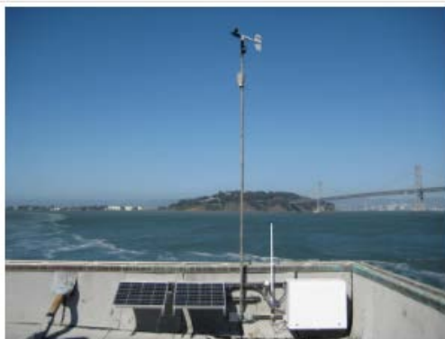
This meteorological station in San Francisco, CA provides wind, air, temperature, barometric pressure, and relative humidity.
