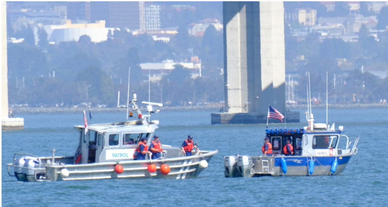
SILVER CHARM and SERVANT set up for a side tow. U.S. Coast Guard Auxiliary photo by COMO Mary Kirkwood.
