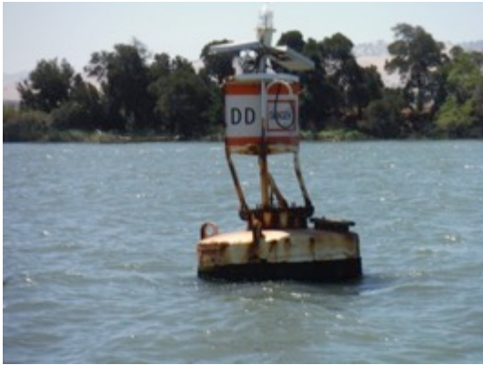
Delta Diablo Outfall Lighted Buoy showing some apparent damage from impact with vessel
